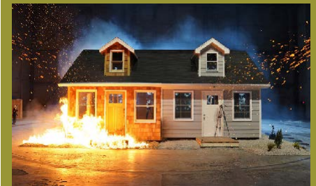
Figure 2b Embers impacting a building: left side with combustible (wood) and the right side with noncombustible (rock) mulch.
